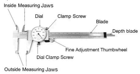
• To read a dial caliper, first note the whole inches and tenths of an inch on the main scale to the left of the reference edge. Then, find the number the dial indicator's needle is pointing to or has just passed, as this represents the hundredths and thousandths of an inch. Add the values from the main scale and the dial for the total measurement.
