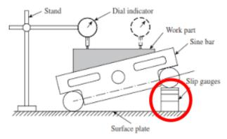
Use the indicator to scan the top of the angled block to determine the offset from left to right.
