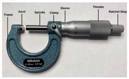
• To read a standard inch micrometer, add the value from the sleeve to the value from the thimble by following these steps: first, read the last full inch and tenths of an inch visible on the sleeve before the thimble. Next, add the value of the quarter marks (0.025") that are visible on the sleeve after the last full number. Finally, add the thousandths of an inch indicated on the thimble by the line that aligns with the horizontal gauge line on the sleeve.
